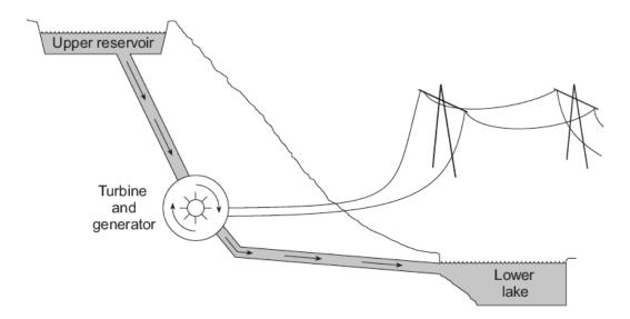
The upper reservoir holds water that flows through the pipes to the lower lake. The electricity that is generated is transmitted along wires that are underground inside the National Park and along wires supported by pylons after that.
